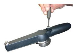
Make sure the movement arm is in-line with the wrench centerline. If the pushrod is off to one side the wrench may not calibrate in one direction or the other (see Fig. 5 and 6 below). The pushrod must also be perpendicular to the top plate or non-linear results may occur (Fig. 7).
